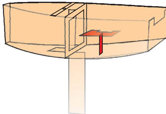
9. Insert mast and rudder tube.
